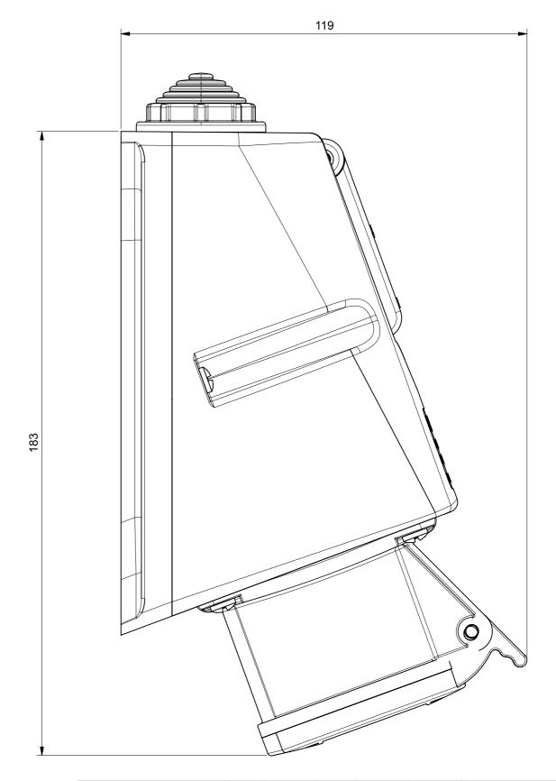
At the end of the law, Format A3 Scale 1:1 Mould N° Drawn SCAME we reserve the ownership of this design may not Tolerances for linear and angular dimensions without indication of specific tolerances: JS13 / UNI EN20286 be copied and transfer it to third parties or competitors Approved CODICE Sheet 1 / 1 DESCRIPTION 4006780 PRESA PARETE COMBI 16A 3P+T - ARGENTINA PARRE - (Bergamo)
